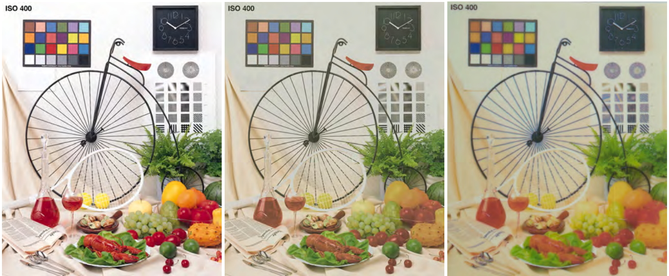
Fig. 11. An image printed with our contoning technique at 720 dpi. From left to right: sRGB original image, color preview after gamut mapping and layer separation, and fabricated result, respectively. The prints have 68 Z-layers, at least 20 of which are white backing layers. (print size (xyz): 2108×2560×68; print time: 9hrs).
