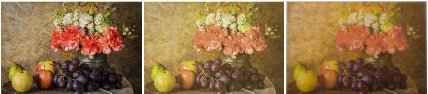
Fig. 12. An image printed with our contoning technique at 720 dpi. From left to right: sRGB original image, color preview after gamut mapping and layer separation, and fabricated result, respectively. The prints have 68 Z-layers, at least 20 of which are white backing layers. (print size (xyz): 3825×2550×68; print time: 15hrs).
