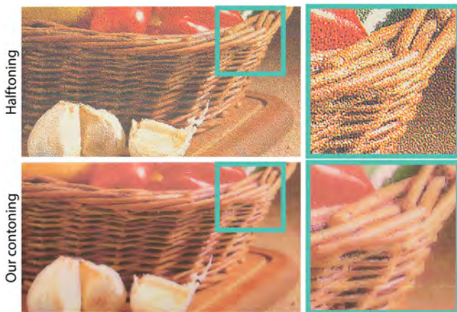
Fig. 17. An image printed with halftoning (top) and contoning (below) at 180 dpi printer resolution (print size (xy) = 2280×1300).
