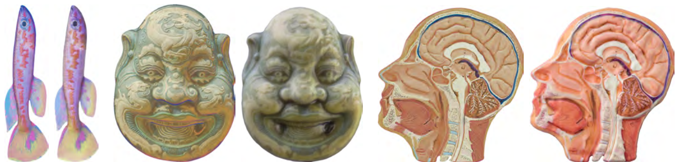
Fig. 13. The preview of our 3D printed models (respective left side of each model) and a photograph of the final print (respective right side of each model). The preview includes the gamut mapping and the layer separation steps. Note that our preview shows an orthogonal top-down view of the 3D printed models, without including the ambient occlusions and/or the blur kernel. Adding these effects for 3D prints can improve the preview significantly.
