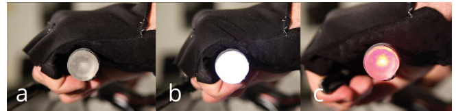
Figure 35. (a) Gloves change the texture to indicate directions; (b) Squeezing one hand to light up the turning light; (c) Squeezing both hand to light up deceleration light.
