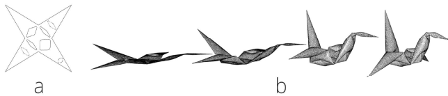
Figure 33. Self-folding crane. (a) The design of hinges. (b) The simulation of the transformation.
