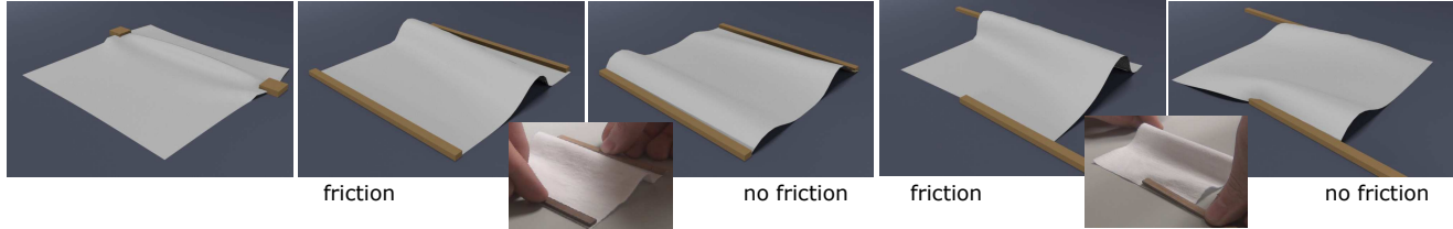
Figure 1: We produce a wrinkle on a piece of cotton (first from left). With internal friction (second and fourth), it becomes a ‘preferred wrinkle’ and arises repeatedly under diverse deformations. Without internal friction (third and fifth), folds and wrinkles show no clear similarity. The insets show real-world deformations for the same experiment.
