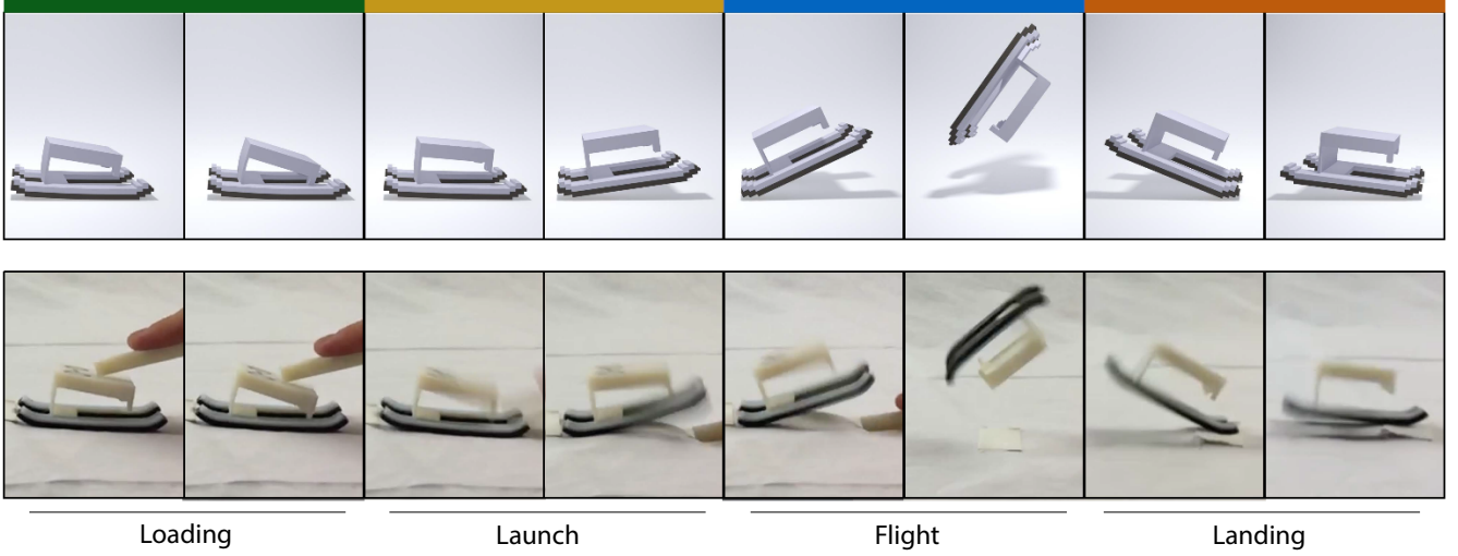
Figure 6: Bottom: the dynamic behavior of a 3D-printed, elastic jumping mechanism in experiment. Top: our DAC-coarsening combined with our BBI impact model generate a simulation that predictively captures this experimental behavior at rates 79X faster than state-of-the-art FEM.
