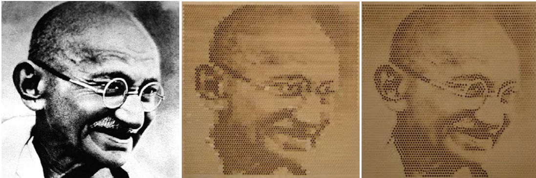
Figure 1: Our system uses an arbitrary image as input (left). Then, it produces a surface with embedded holes such that the shading due to occlusion induces the desired image. We fabricate these surfaces using computer-controlled milling machines. We show that aligning holes with image features improves reproduction quality (right) compared to regular hole pattern (center).
