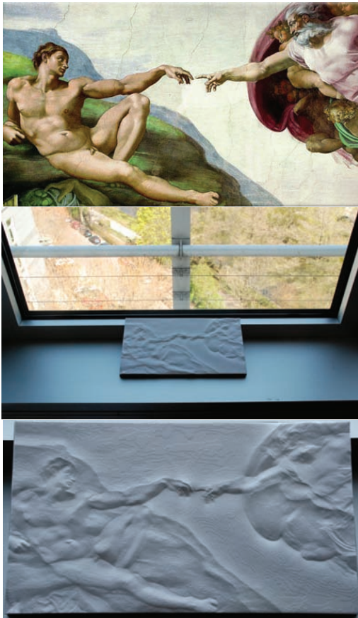
Figure 6: A relief created from the image in the top row. The illumination for capturing the image is created by simply putting the relief close to a window (middle row), showing that the images created by the reliefs are not very sensitive to the particular illumination setting.
