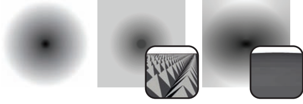
Figure 3: Creation of reliefs for the canonical “impossible” image (left) from [Horn et al. 1993]: using pyramids we could create a qualitatively perfect reconstruction of the image (i.e. the gradient images are almost identical), albeit at the expense of pronounced pyramid, which cause extreme dependence on perfect viewing and illumination conditions (center). We suggest to optimize the heights of vertices and impose smoothness constraints and arrive at the reconstruction shown on the right (which is worse based on comparing the image gradients). The insets show a perspective view over the surface, illustrating the clearly visible pyramids in the center image and no visible variation in heights in the right image.
