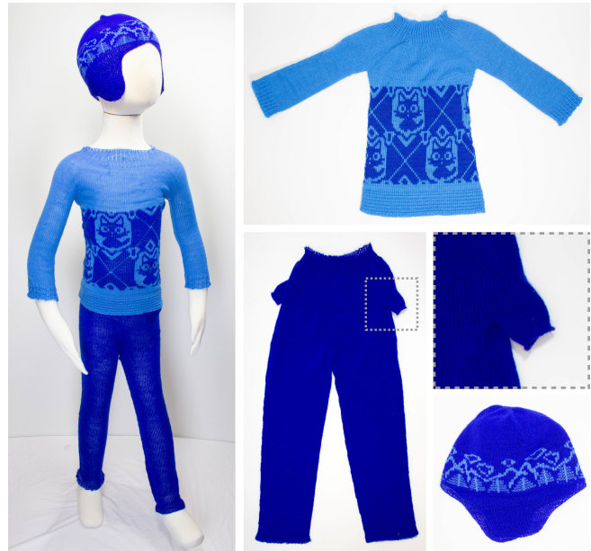
Fig. 13. Our larger examples on a 4-foot boy mannequin, together with top-down views of the individual garment pieces and a zoom on one of the in-seam pockets of the trousers which are knit as inside-out tubular structures merging with the body.
