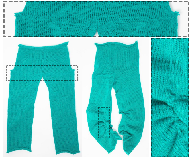
Fig. 17. Example of knitting failures due to failing needle transfers: the left example failed at large decreases above the crotch due to non-ideal schedule alignments; the right example had catastrophic failures due to overlapping loop transfers during shaping transfers.
