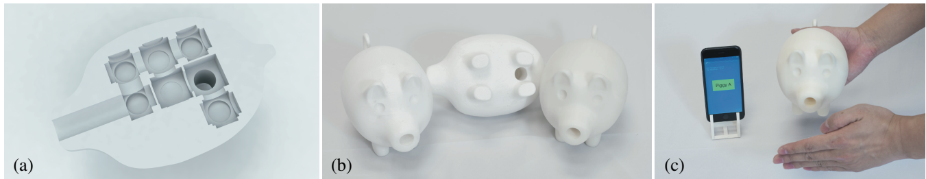
Figure 1: Acoustic Tagging. By optimizing the structure of primitives (a), we control the acoustic response of an object when it is tapped (c) and thereby tag the object acoustically. Given three objects with identical shapes (b), we can use a smartphone to read the acoustic tags in realtime, by recording and analyzing the tapping sound, and thereby identify each object.
