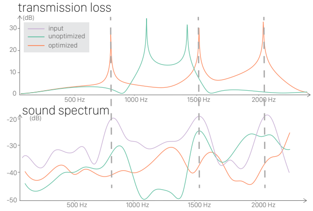
Figure 11: Engine Muffler. We compare an unoptimized muffler and an optimized one. The three noisy peaks are suppressed to lower levels with the optimized muffler.
