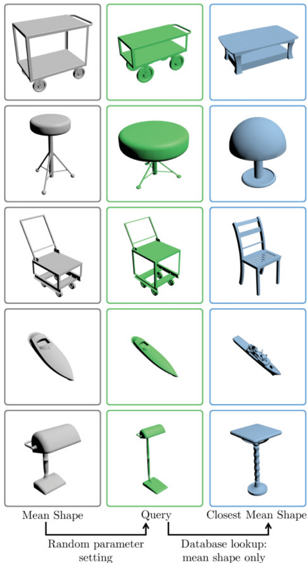
Fig. 10. Demonstration of query failures when representation only consists of the mean shape. From left to right: the mean shape of some parametric models in our database, query shape given by a random parameter setting of each parametric model, and the closest mean shape retrieved from the database. Since changes in parameter settings significantly alter the geometry, the closest mean shapes are usually not from the parametric models that originate the queries.
