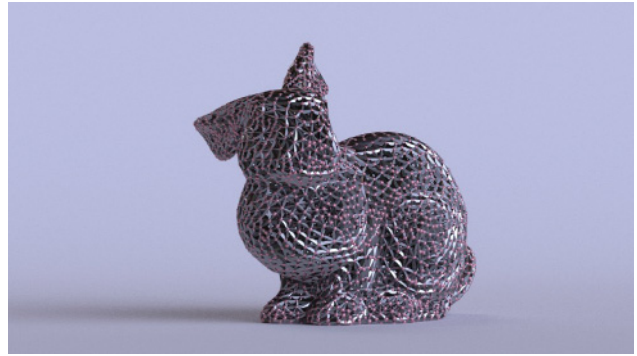
Fig. 11. Still from an Implicit Springs simulation of the Stanford bunny. The bunny consists of 36,976 vertices and 220,147 springs, which can be simulated by Simit on a GPU at 12 frames per second. Only surface vertices and springs are shown. The Simit code is only 93 lines, which includes a conjugate gradient solver implementation.
