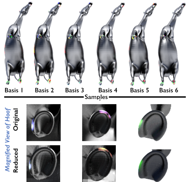
Figure 5: Top Row: Six (of 108) basis vectors computed for a Drop Tested horse. Note that our basis vectors consist of sparse collections of contact forces (zoom in). Bottom Row: Comparison of original force samples to their reconstructions in the basis. Here we focus only on the contact area, forces are zero elsewhere in both the original sample and its reduced representation. Colors represent the x (red), y (green) and z (blue) components of the applied force.
