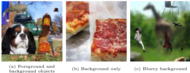
Fig. 4. Sample data. Example frames from our dataset. (a) Our data consists of pasted foreground objects using segmentation from PASCAL VOC [25] and background from MS COCO dataset [26]. (b) To ensure our network learns global motion, the second part of our dataset only has background moving. (c) To ensure low contrast texture is well-represented, we include data with the background blurred. We add another two parts with the same specification as (b) and (c) with background motion removed so that the network learns the changes that are due to noise only.
