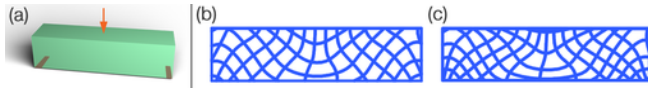
Fig. 7. Varying \beta to control truss spacing for the bar with fixed ends problem: the problem domain and boundary conditions (a), a slice of the truss extracted by setting \beta = 1 , thus preferring regular spacing over orthogonality of the parametrization (b), and the same slice with \beta = 0.1 , which favours parameter orthogonality (c).
