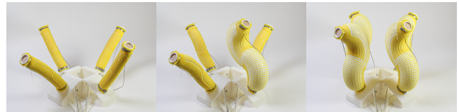
Figure 12: Interactive actuator: the integrated swept frequency capacitive sensing detects human's touch and the actuators activate with shape changes.
