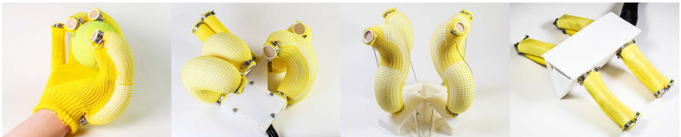
Figure 1: Example applications of machine-knitted pneumatic actuators: from left to right, assistive glove, soft hand, interactive robot, and pneumatic quadrupedal robot.
