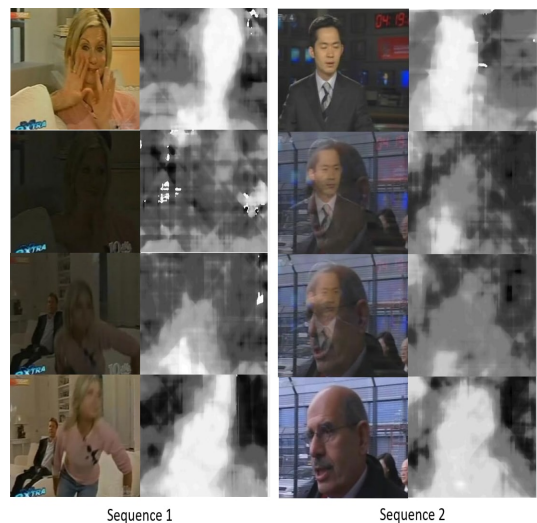
Fig. 2. A figure illustrating the importance of shot boundary detection during 2D-to-3D conversion. Here, we show consecutive frames from two sequences. For each frame we show its original RGB image (left) and the corresponding disparity map (right) as estimated by the 2D-to-3D conversion technique of Bae et al. [7]. The disparity maps is a gray-scale image where white represents objects close to the screen. Note how the disparity captures the humans outlines before and after transitions (first and last frame). During gradual transition, however, the outline is severely destroyed. This is because gradual transitions violate the single layer model used by many video processing techniques. Hence, it is desirable to detect such gradual transitions and to give them a special treatment during post-processing. For this, shot boundary detection is essential.
