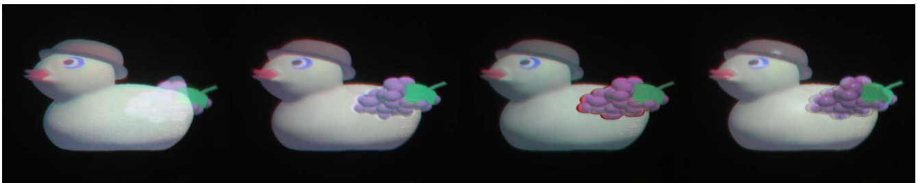
Figure 1: Illustration of the steps of our light field decomposition. (1) volumetric rendering, (2) view-independent and (3) view-dependent occlusion culling, (4) view-dependent rendering on parallax type layer. Photographs are taken from our multi-layered display prototype.
