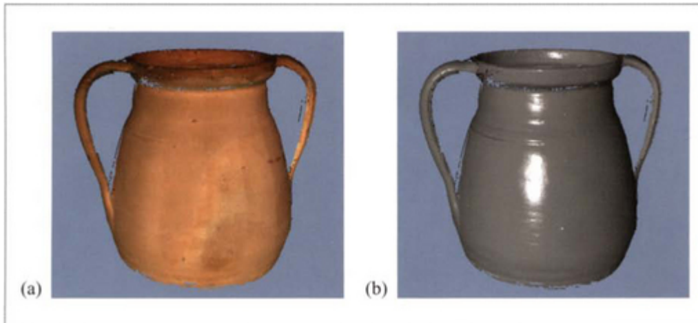
Figure 3.17 Clay pot reconstructed from 15 rotary views (384,492 surfels). Lambertian texture (a) and synthetic Phong texture (b) for showing geometric detail. The Lambertian texture exhibits stripe artifacts due to specular reflection of the clay surface.
