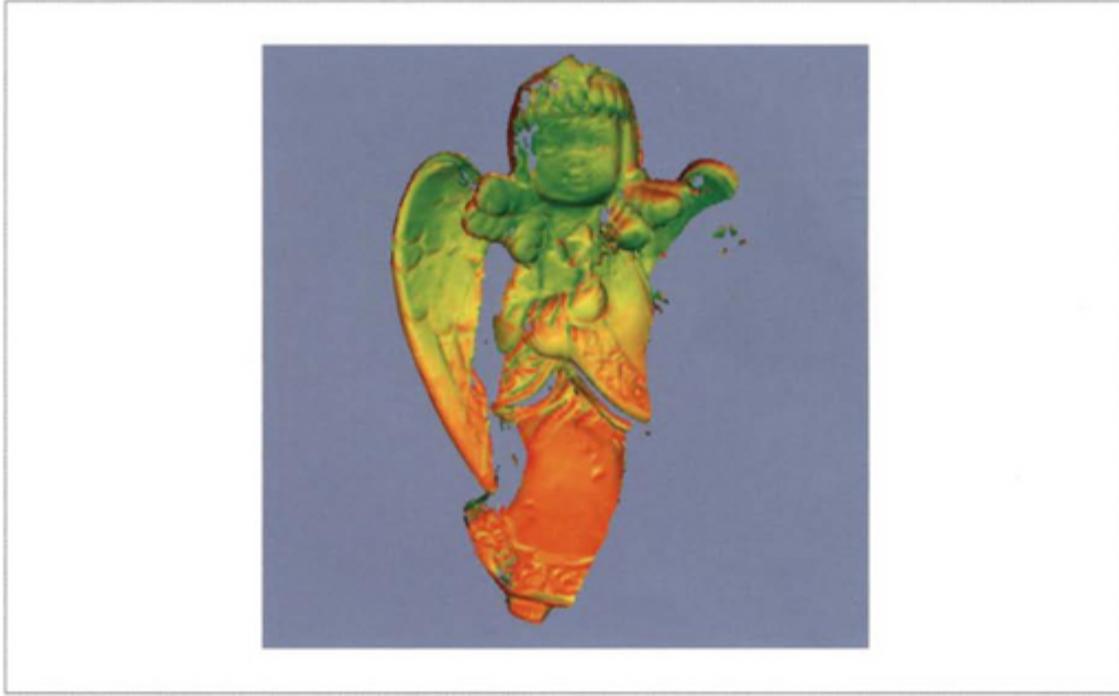
Figure 3.11 Single-ring reconstruction colorized by the ray skew for verification of calibration quality. Red means small skew; surfels with ray skew larger than 0.6 mm (outliers) have already been removed.
