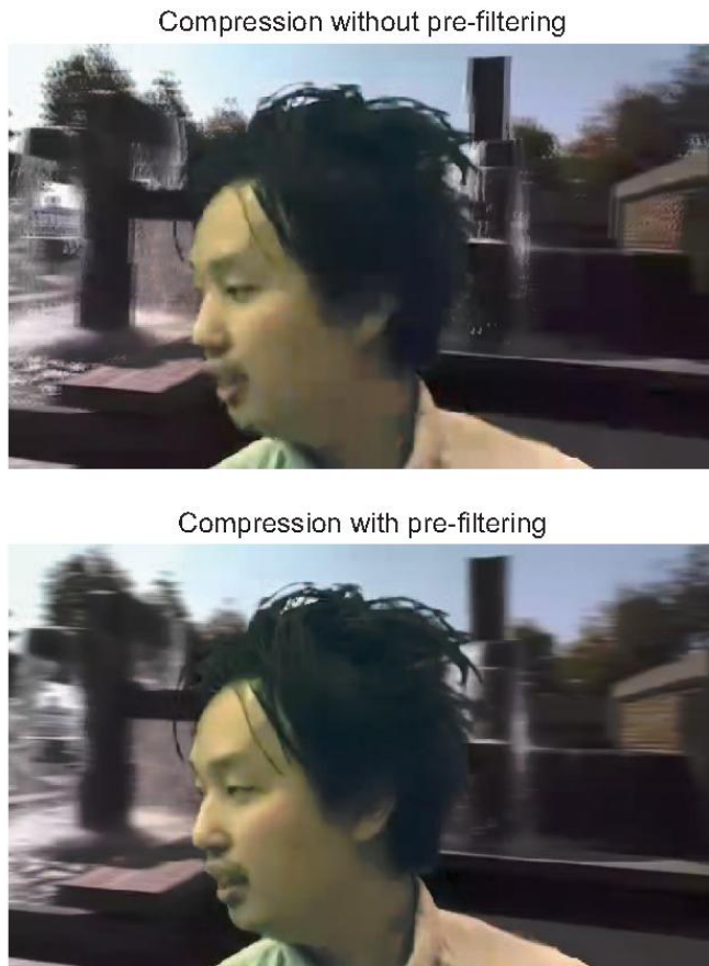
Fig. 3. Comparison of compressed frames of a video sequence with and without pre-filtering. The images show simulated views of a multi-view 3D display. The version without pre-filtering at the top shows stronger blocking artifacts than the version with pre-filtering at the bottom. In addition, pre-filtering avoids ghosting artifacts, which appear without pre-filtering in the background in the top image.
