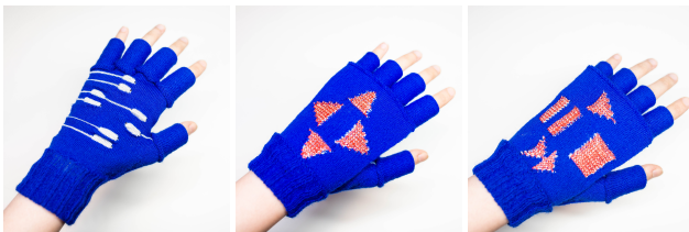
Figure 16: Glove controller: left, conductive traces are added to existing knitted glove design; middle and right, glove with different controller designs.
