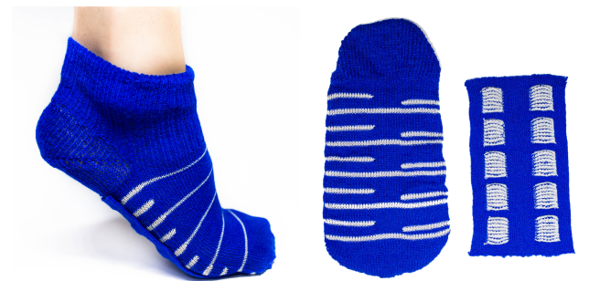
Figure 17: Tactile sensing socks
