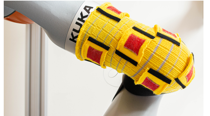
Figure 20: Kuka with knitted sensing covering: grey is the conductive yarn and red rectangles are sensors.
