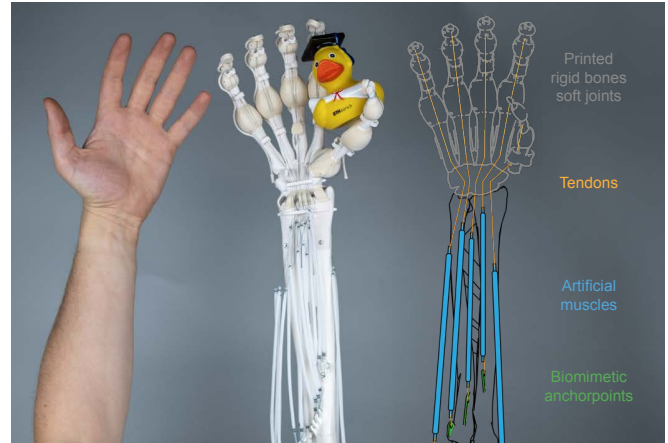
Fig. 1. Pneumatic musculoskeletal hand and forearm. Inspired by the human anatomy, we printed a musculoskeletal hand and forearm. The soft-rigid hybrid hand is printed in a single process and does not need assembly apart from attaching thin McKibben muscles for actuation. We replicated the anchor points and muscle lengths from the biological inspiration.
