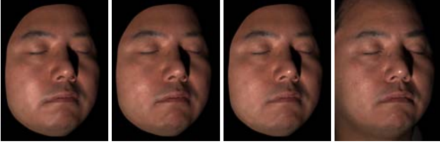
Figure 6: Torrance-Sparrow model and (from left to right) (a) only diffuse normal map; (b) one diffuse and one global micro-normal map for specular reflection; (c) one diffuse and per-view micro-normal maps; (d) input photograph. Method (c) most accurately reproduces the specular highlights of the input image.
