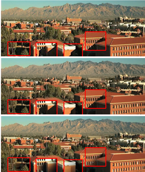
Figure 11: Closeup of a frame in the Arizona sequence. Top: Original image. Middle: FTLV reconstruction with 14.5% RMS error. Bottom: PCA reconstruction with the same error using five terms plus the mean. Note the blurry shadows in the PCA reconstruction.
