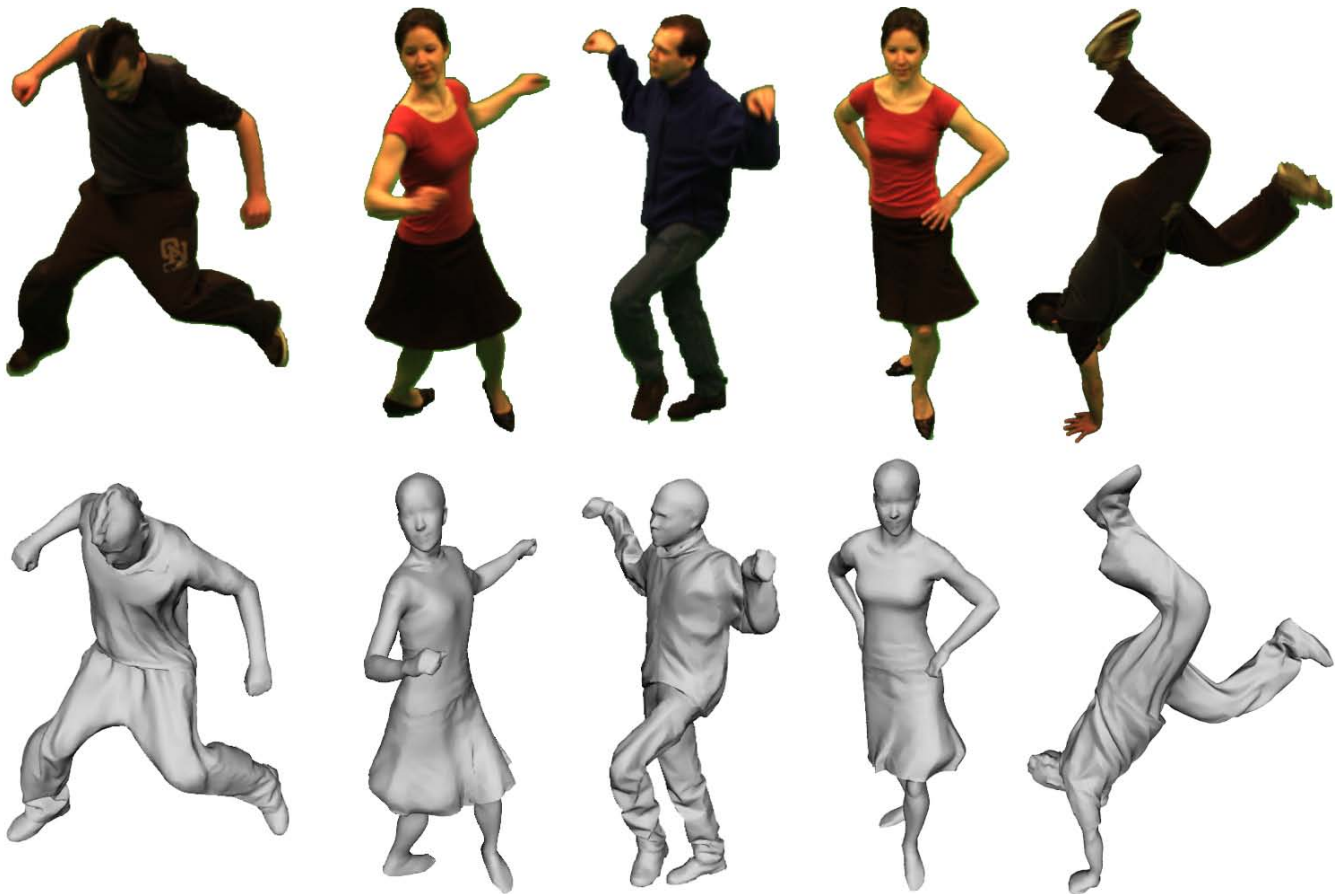
Figure 8: Background-subtracted video frames (top) and the corresponding recovered shapes (bottom) for three subjects in five sequences.
