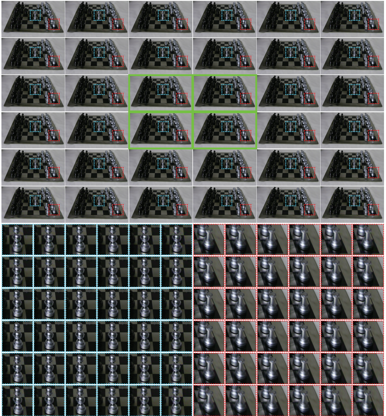
Figure 10: The top image array corresponds to a small light field created from four images marked in green. The small insets below present magnified fragments of the reconstructed images. Please refer to the electronic version of the paper to see the images in a zoomed-in version. The input images come from "The Stanford Light Field Archive" ( http://lightfield.stanford.edu/lfs.html ).
