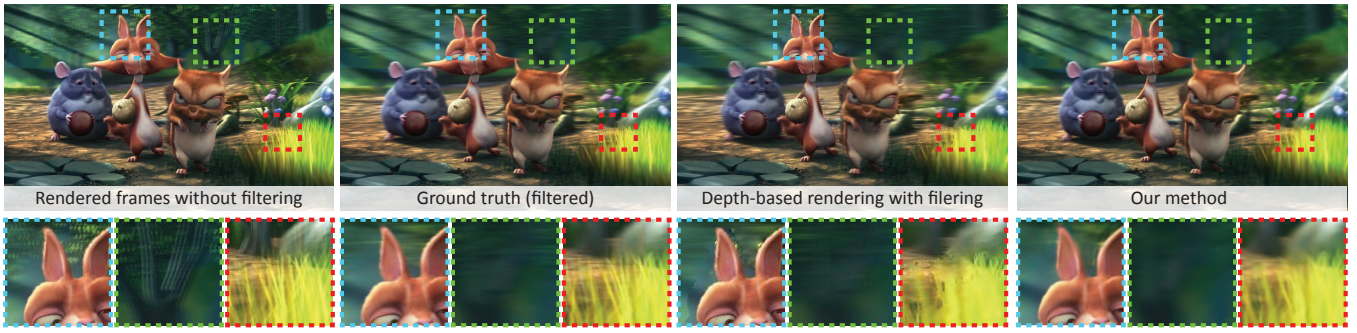
Figure 4: Comparison of different content creation approaches for automultiscopic display. When each frame is rendered, but antialiasing is not applied a significant ghosting is visible for objects located further from the screen plane (green insets). These artifacts can be removed when the content is properly filtered but this requires rendering hundreds of views. Image-based techniques combined with filtering can produce good results for many cases, but also can introduce significant artifacts when depth estimation fails (red insets). Our method produces results similar to rendering with filtering, but at cost similar to real-time image-based techniques. ("Big Buck Bunny" © by Blender Foundation)
