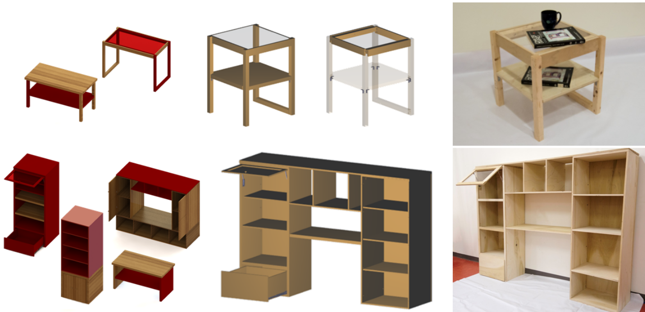
Figure 13: From left to right: input designs, models created using the system, and fabricated results. We highlight the connecting elements on the first model by making all principal elements semi-transparent.
