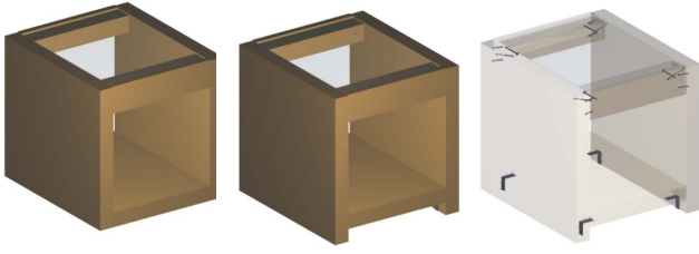
Figure 10: An example of changing parameters to fit connectors. From left to right: the bottom shelf snapped to the bottom of the table, the resulting configuration of the model after the connecting step, and the visualization of the connectors (principal elements are made semi-transparent). Notice that, in order to connect the bottom shelf to the table legs, the system raises the shelf above the ground to leave room for l-brackets.
