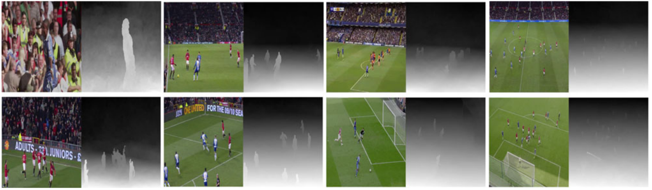
Fig. 9. Depth estimation for different types of shots using our method. Our method handles a wide variety of shots including Close-ups (e.g., top, left-most), Medium Shots (e.g., bottom, left-most), Bird's Eye View (e.g., bottom, right-most) and Long Shots (e.g., top, right-most).
