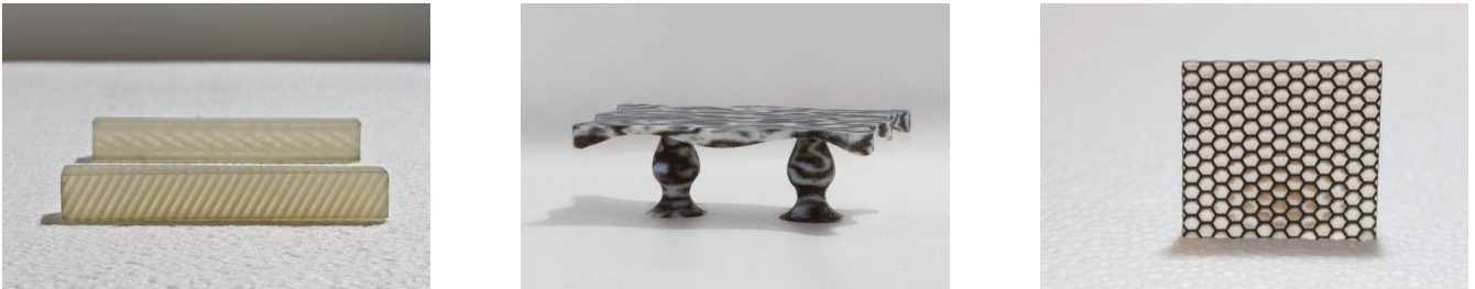
Figure 8. Left: procedurally defined materials with anisotropic mechanical properties. Center: Marble-like material generated using Perlin noise. Right: Procedurally defined and fully parameterized aspherical microlens array with baffles.
