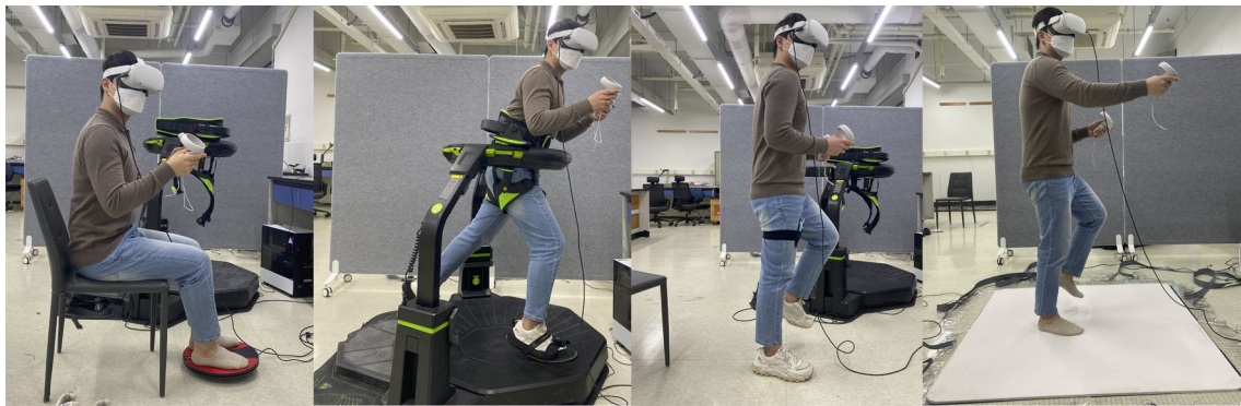
Fig. 4 (Left to right) Foot mouse, treadmill, leg strap, and proposed Seamless-walk systems. Each picture demonstrates how each locomotion method is used
