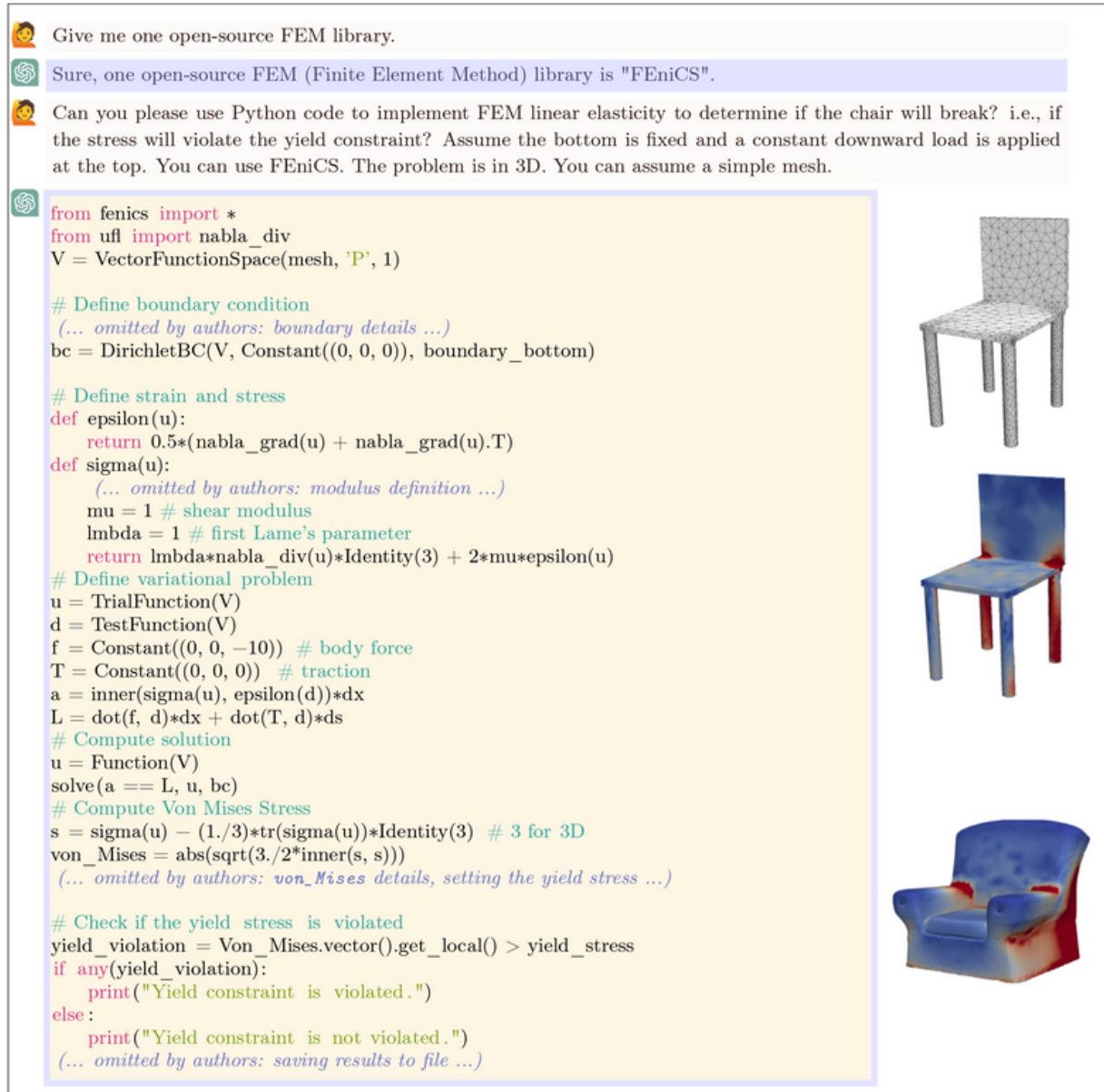
Figure E33. Finite element analysis for chair mechanics. GPT-4 determines if the chair will break by performing FEM-based stress analysis. In images, the top chair analyzed is designed by GPT-4 in Figure B10 with von Mises stress displayed from blue (zero) to a maximal value (red). A second chair with mesh from an external source is analyzed using the same code.
