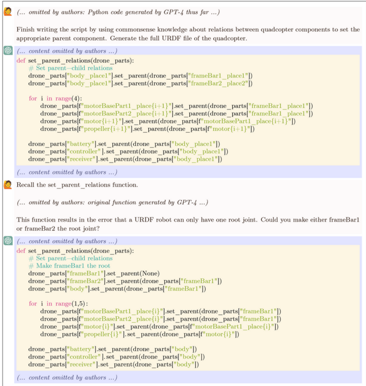
Figure 13. Constructing relations between quadcopter links. After creating and placing links in the appropriate positions, GPT-4 must infer parent-child relations that are not available in the OpenJSCAD design to complete the Universal Robot Description Format (URDF) representation. In its first attempt, it produces an invalid file because only one of the frame bars can be the root joint. However, GPT-4 demonstrates an understanding of how the motor, motor base, and propeller should be connected and that the main body contains the battery, controller, and receiver.
