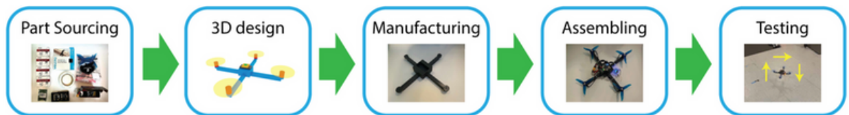
Figure 7. The quadcopter design process using GPT-4. The process involves sourcing parts, creating a 3D design, manufacturing, assembling, and testing the quadcopter. We successfully manufactured a working quadcopter.
