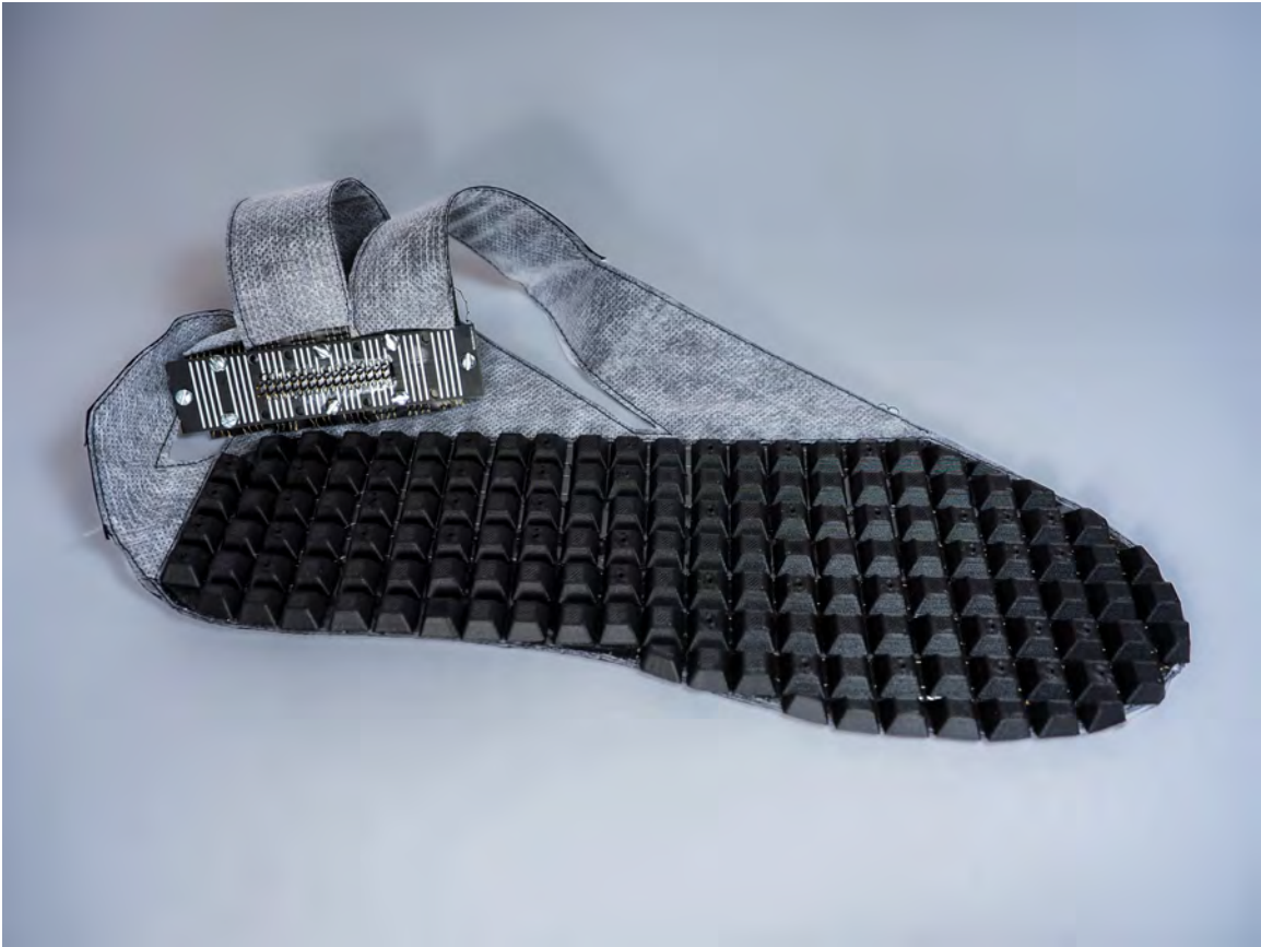
Figure 4-4: Images of our multi-modal tactile sensing insole.
