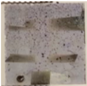
Figure 6-1: One of the two working devices. Of the four pixels visible here (not counting the base contact at the bottom), one of them functioned at 0.08% efficiency and the other three did not work (were shorted). Observe that the aluminum deposition pattern is the areas not covered by the shadow mask pattern depicted in Figure 3-4
