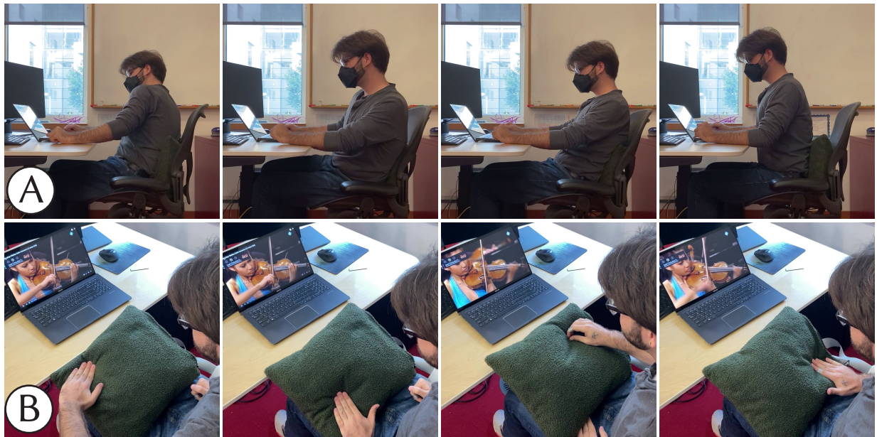
Figure 3.11: Tactile Sensing Pillow: Used for (A) Posture monitoring, from left to right: leaning right, leaning left, leaning back, sitting up straight and (B) Remote Control, from left to right: Play, Pause, Volume Up, Volume Down.
