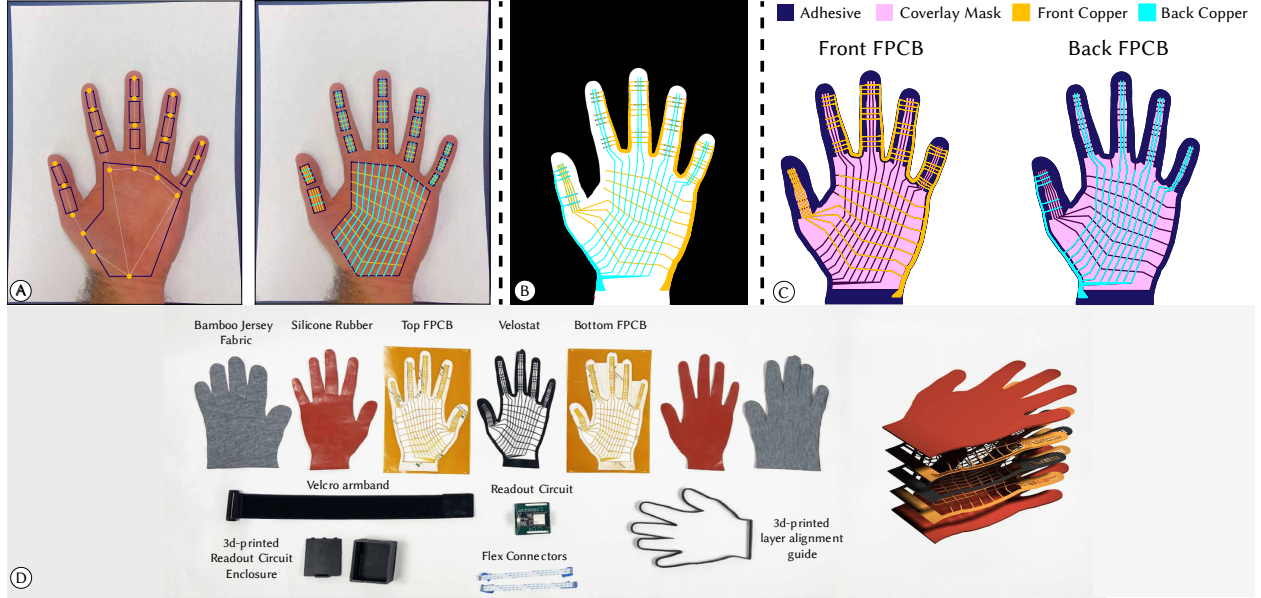
Figure 4.2: Automated FPCB design and sensor assembly. (A) Sensing regions are detected and orthogonally arranged electrodes are generated within them. (B) The binary mask of the hand is used to extract its contour, which serves to connect electrodes across neighboring regions. (C) Supporting layers of the PCB are generated and used to create Gerber files which can be sent directly to PCB manufacturers. (D) Sensor assembly using materials totaling under $130 dollars by sandwiching 5 layers together with pressure-sensitive adhesive.
