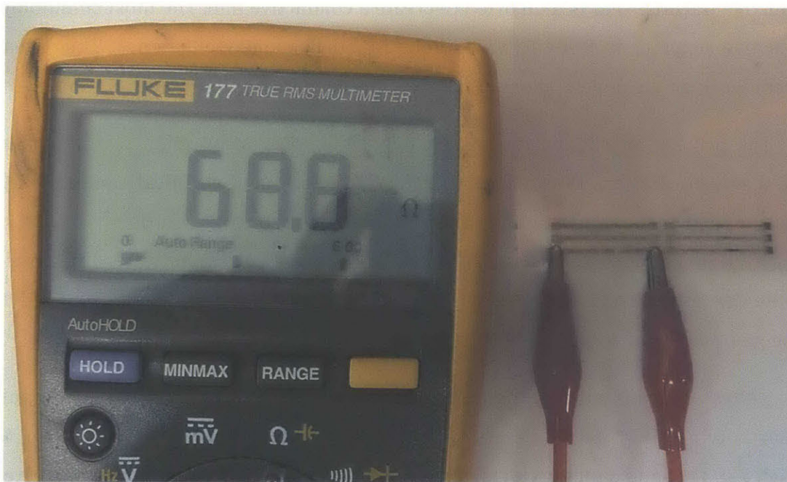
Figure 34. Printed silver nanoparticle conductive traces. The traces have a resistivity of about 50 ohms/cm. The sample was sintered in an oven at a temperature of 100°C for one hour.
