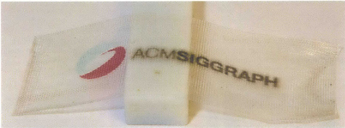
Figure 31. 3D printed thin polymer fabric with a 90° grid pattern. Colored symbols and letters were added to show the potential for fabricating elaborate patterns. The fabric is flexible and easily conforms to surfaces. The fabric is about 500 microns thick.
