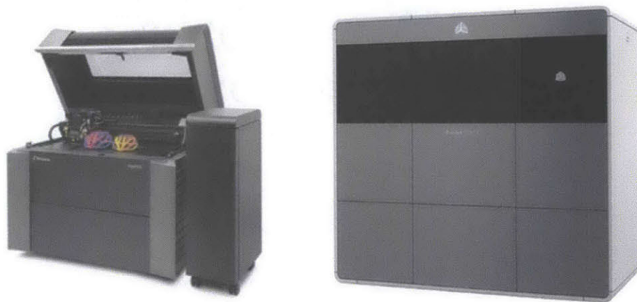
Figure 2. Objet500 Connex3 and 3D Systems ProJet 5500x multi-material 3D printers. The Objet500 features three printheads and allows color printing. The price of these printers is in the $300k range.
