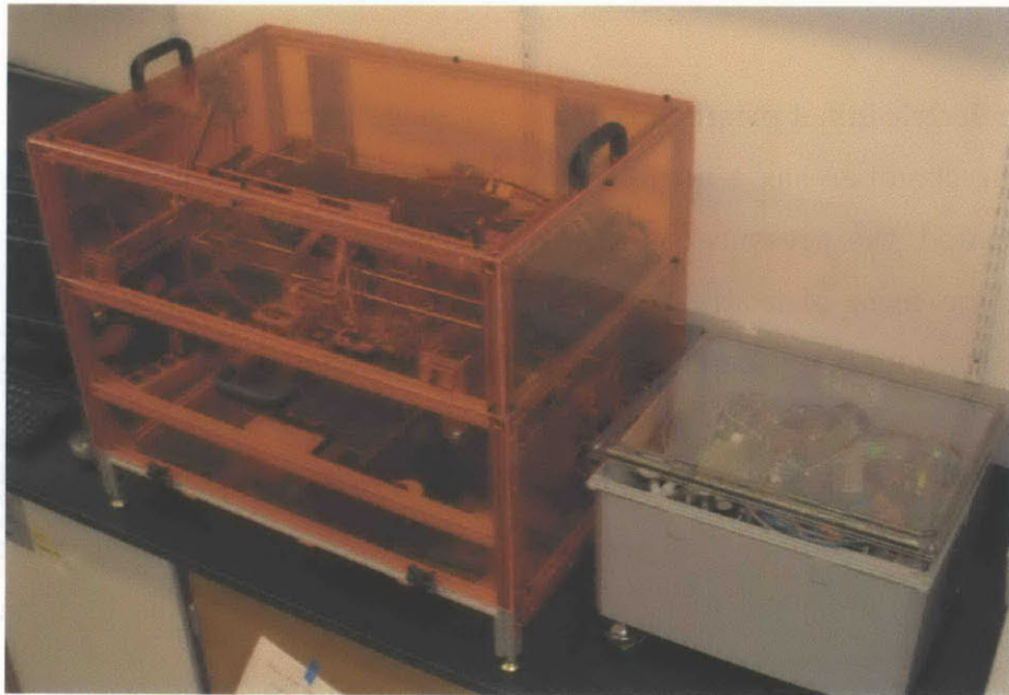
Figure 14. Fully encased MiniFab 3D printer. The cover protects users from the UV curing light.
