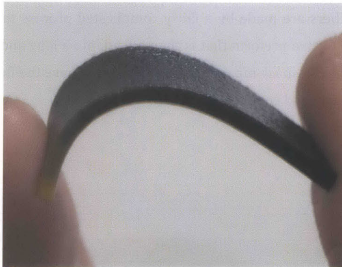
Figure 20. A 3D printed FGM slab with a rigid, ABS-like material, RIG-3 and a flexible material, ELA-4. The materials are linearly graded from left to right: 0% RIG-3 and 100% ELA-4 in the left end to 100% RIG-3 and 0% ELA-4 in the right end. Note that the left end exhibits considerable flexibility relative to the right end.
