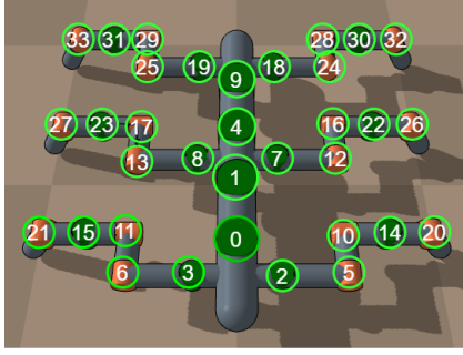
Figure 1.1: Graph Structure and Neural Network Modules of the 6 Leg Centipede. Left: The robot’s joints are labeled numerically and circled. Right: The joints form the nodes and the links are the edges. The subset of joints that form each leg module are circled in red, while those that comprise each body module are circled in blue. Neural network modules are denoted as \mathbf{W}_k^i , where k refers to the type, e.g. all leg modules are type 0, and i denotes different instances of the same module type.
