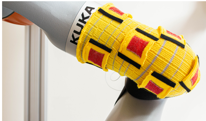
Figure 3-11: A robot arm (KUKA) with knitted sensing covering. Conformal robot arm sleeve with sensors in red and conductive traces in grey.
