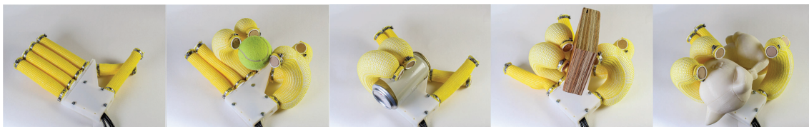
Figure 5-12: Soft hand. The actuation of each finger is individually addressable by a pneumatic valve system, allowing us to realize a variety of hand poses and grasp objects with different shapes, textures, and weights.
