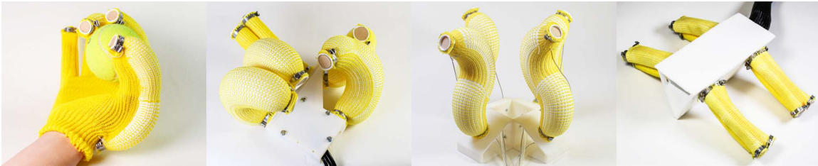
Figure 5-1: Example applications of machine-knitted pneumatic actuators. Example applications include assistive glove, soft hand, interactive robot, and pneumatic quadrupedal robot.
