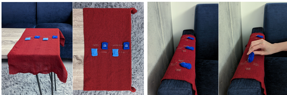
Figure 6-17: Furniture covering. Leveraging digital design and fabrication pipeline, MagKnitic can be integrated into furniture coverings, including table cloth, and sofa coverings, for diverse user interactions with passive haptic feedback. Using scenarios include tangible and interactive task checklists, ubiquitous user input interfaces, and so on.
