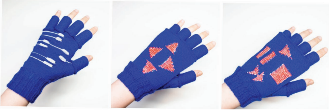
Figure 3-9: Interactive wearables. Conductive traces are added to existing knitted glove design for gloves with different controller designs.
