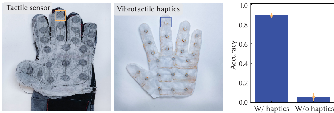
Figure 7-15: Transfer physical tactile interaction for one person. Left: Photograph of an outer sensing glove to capture tactile cues and an inner haptic glove to transfer tactile cues under tactile occlusion. Right: Accuracy of classification of single contact points under tactile occlusion, with and without the haptic feedback. Error bars indicate the standard deviations (SD) across measurements.
