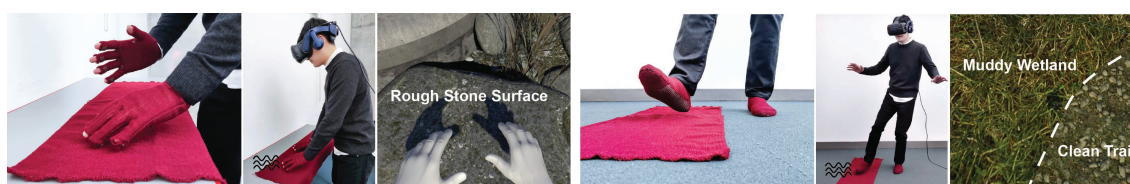
Figure 6-18: Interactive wearables for AR/VR. Potential application of passive yet interactive gloves and socks for surface textures rendering in VR environments.
