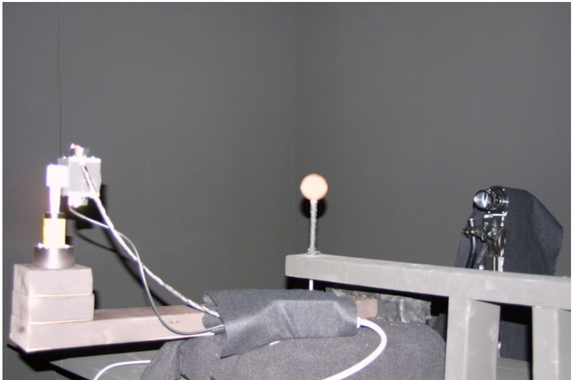
Figure 3-1: A photograph of my high-speed BRDF measurement gantry.
