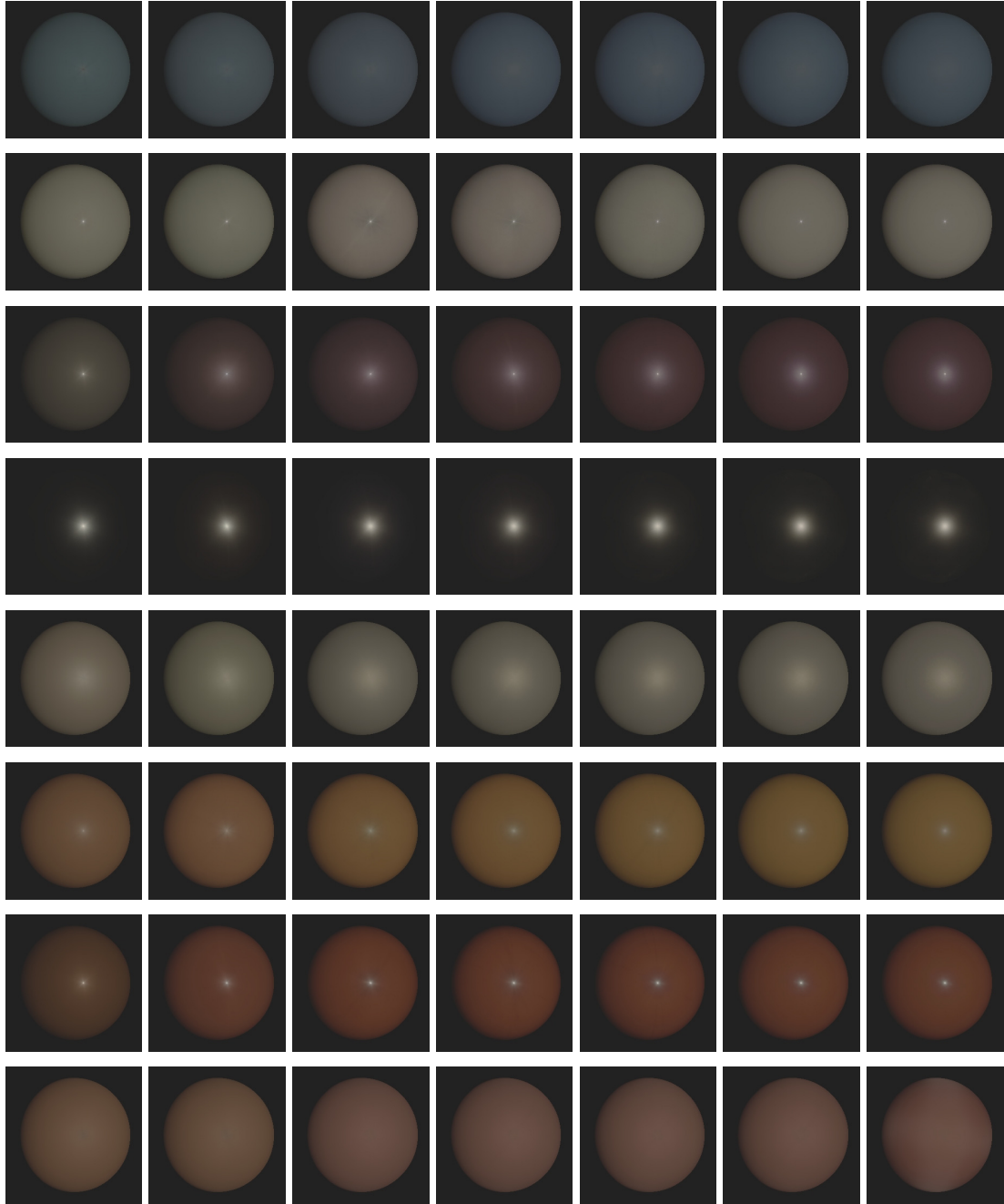
Figure 4-3: Reconstruction of different BRDFs from principal components in order (left to right) of increasing number of components: 5, 10, 20, 30, 45, 60, and all. Each row represents one BRDF: blue rubber, alumina oxide, violet acrylic, nickel, pearl paint, yellow matte plastic, red phenolic, and pink fabric.
