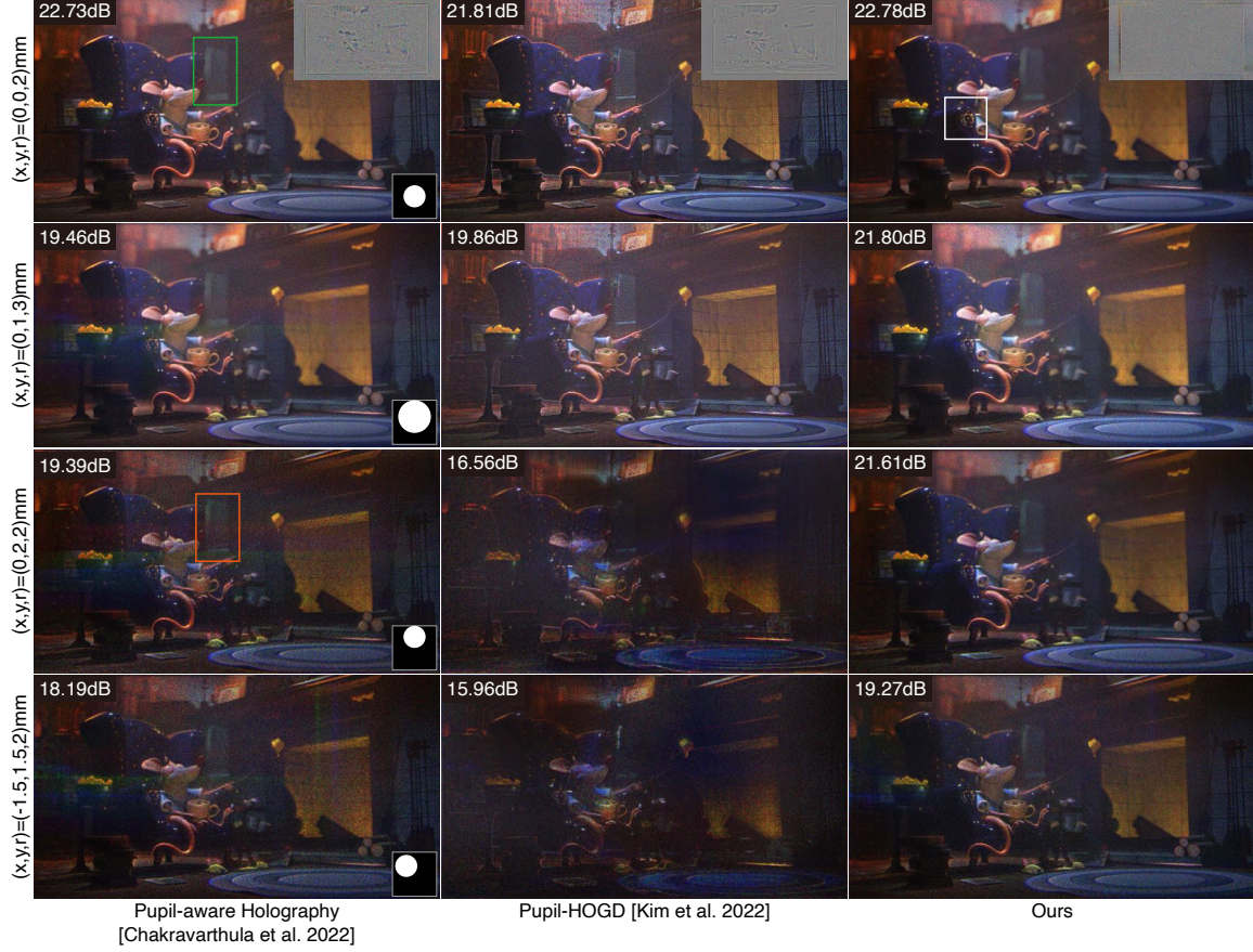
Figure 6-7: Comparison of 3D CGH algorithms on experimental results captured at various pupil locations and sizes. The bottom right corners in column 1 images mark the pupil position and size used to capture the results in the respective row. The numbers indicate the PSNR with respect to the target image. Source image: “Mr. Elephant”, reproduced under terms of the CC-BY-ND license, Copyright 2017, by Glenn Melenhorst, published with the author’s permission.
