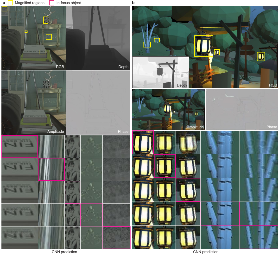
Figure 4-7: Evaluation of tensor holography CNN on additional computer-rendered scenes. CNN prediction of amplitude and phase along with focused reconstructions for holograms of a , a living room scene from the DeepFocus dataset [258] and b , a night landscape scene from the Stanford light field dataset [200].
