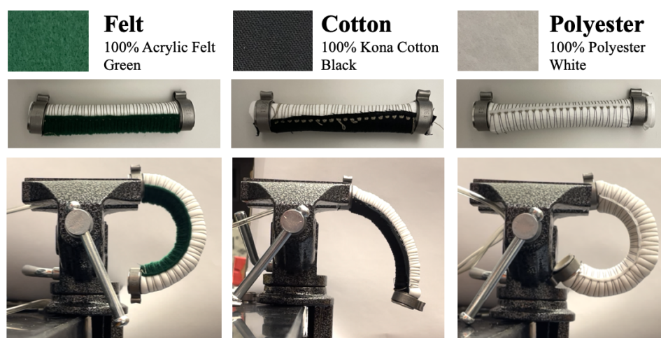
Figure 9: Three different fabrics (cotton, felt, polyester) integrated into embroidered actuators. The displacement of the actuators at a pressure of 30psi can be seen.
